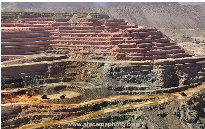
Copper<sup>1</sup> can be found throughout the earth's crust, but is worth extracting when there is about 2 kg of copper per 1,000 kg of ore. Ninety per cent of copper ore is mined using the open pit method<sup>2</sup> which is an excavation or cut made at the surface of the ground for the purpose of extracting ore. To expose and mine the ore, it is generally necessary to excavate large quantities of waste rock.<sup>3</sup>
